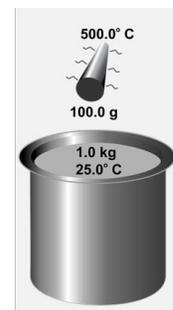
The specific heat capacity of iron is 0.11 cal/g°C, and for water, 4.18 cal/g°C.
